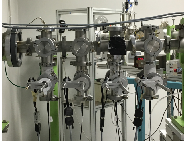
Figure 10: The {}^4\text{PrOB}\epsilon\text{aM} system installed on the research beamline of the TR24 cyclotron in Strasbourg. Four UniBEaM beam profilers are visible.
