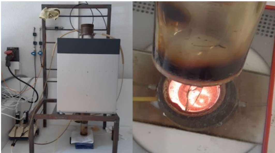
Fig. 1: The atmosphere controlled oven at IRAP for heating under reducing conditions [11].
