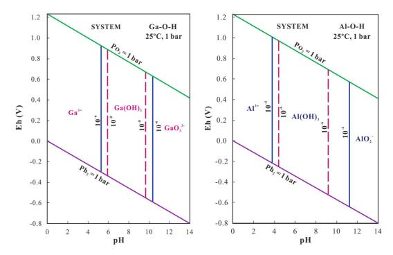
**Figure 3.** Eh-pH diagram of Ga (a) and Al (b). The assumed activities for the dissolved species are  $10^{-8}$  for Ga, and for  $10^{-4}$ .  $^{-6}$  Al (Brookins, 1988).
