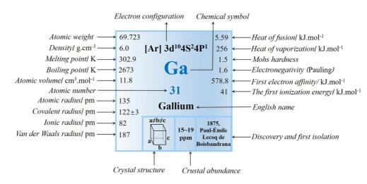
Figure 1. The physicochemical characteristics of Ga.
