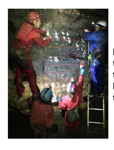
Fig. 9 : Installation of the optic fiber in a vertical plane for water level detection inside the cavity.
