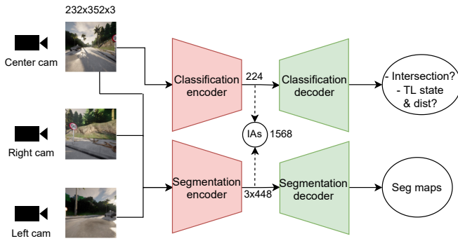
Fig. 2: Feature extraction from RGB camera images for the visual subsystem. Two encoder-decoder networks are pretrained on segmentation, classifications and regression tasks. Classifications and regression are performed on the center image while all three images are segmented. After training, the visual encoders serve as fixed feature extractors with frozen weights. For the DRL backbone training, both encoder outputs are concatenated and sent to the memory buffer as input to DRL. Both encoders are Efficientnet-b1. The segmentation decoder is fully convolutional, and the classification decoder is an MLP with several outputs.
