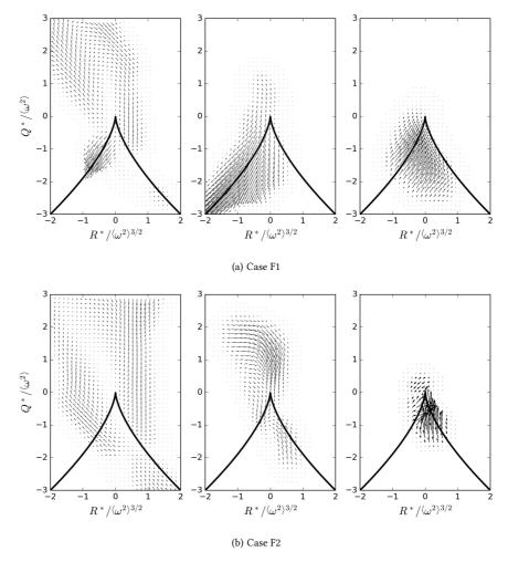
Figure 7. Conditional mean vectors in the  $(R^*,Q^*)$  invariants plane for case F1 (a) and case F2 (b). Left column: c < 0.01 (fresh reactants), middle column: 0.01 < c < 0.50, right column: 0.50 < c < 0.95.
