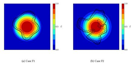
Figure 2. Field (in colors) of the averaged progress variable  $\overline{c}$  at  $t^*=3.0$  together with three instantaneous progress variable iso-lines issued from a cut-plane of the computational domain (solid line: c=0.01, dot-dashed line: c=0.50, dashed line: c=0.95). Case F1 on the left (a) and case F2 on the right (b).
