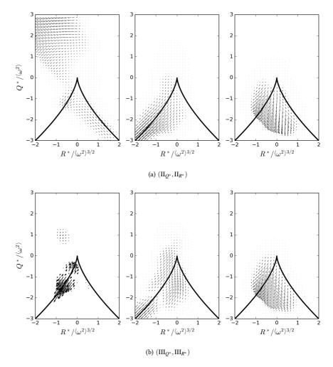
Figure 9. Contributions of the pressure Hessian term II (a) and baroclinic term III (b) to the CMV in the  $(R^*,Q^*)$  plane (case F1). Left column: c < 0.01 (fresh reactants), middle column: 0.01 < c < 0.50, right column: 0.50 < c < 0.95.
