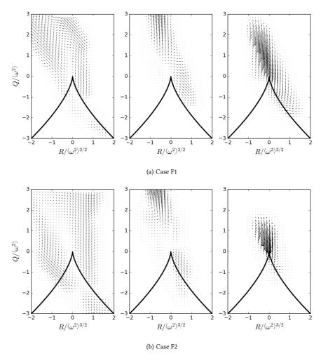
Figure 12. Conditional mean vectors in the (R,Q) invariants plane for case F1 (a) and case F2 (b). Left column: c < 0.01 (fresh reactants), middle column: 0.01 < c < 0.50, right column: 0.50 < c < 0.95.
