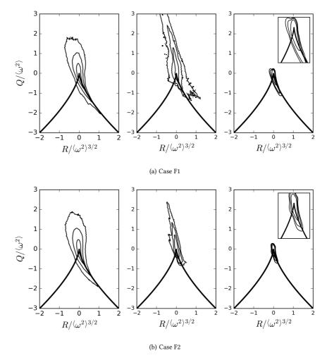
Figure 10. Iso-contours of the joint PDF of the third and second invariants (R,Q) of the VGT in (a) case F1 and (b) case F2. Left column: fresh reactants (c < 0.01), middle: flame region (0.01 < c < 0.95), right: burnt gases (c > 0.95). The three thin lines are the iso-contours of  $\log_{10}(\text{JPDF})$  equals to -2.0, -1.0, and 0.0.
