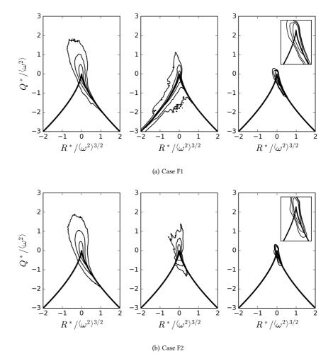
Figure 6. Iso-contours of the joint PDF of the third and second invariants ( $R^*$ , $Q^*$ ) of the traceless VGT in case F1 (a) and case F2 (b). Left column: fresh reactants (c < 0.01), middle: flame region (0.01 < c < 0.95), right: burnt gases (c > 0.95). The three thin lines are the iso-contours of  $\log_{10}(\text{JPDF})$  equals to -2.0, -1.0, and 0.0.
