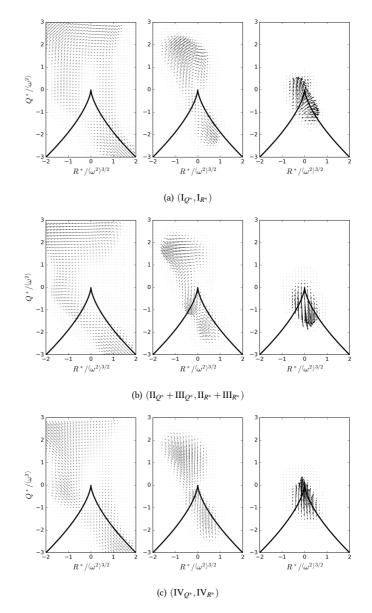
Figure 15. Contributions I (a), II+III (b), and IV (c) to the CMV as given by the LEE for  $Q^*$  and  $R^*$  (case F2). Left column: c < 0.01 (fresh reactants), middle column: 0.01 < c < 0.50, right column: 0.50 < c < 0.95.
