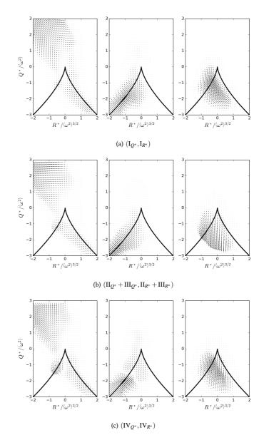
Figure 8. Contributions I (a), II+III (b), and IV (c) to the CMV as given by the LEE for  $Q^*$  and  $R^*$  (case F1). Left column: c < 0.01 (fresh reactants), middle column: 0.01 < c < 0.50, right column: 0.50 < c < 0.95.
