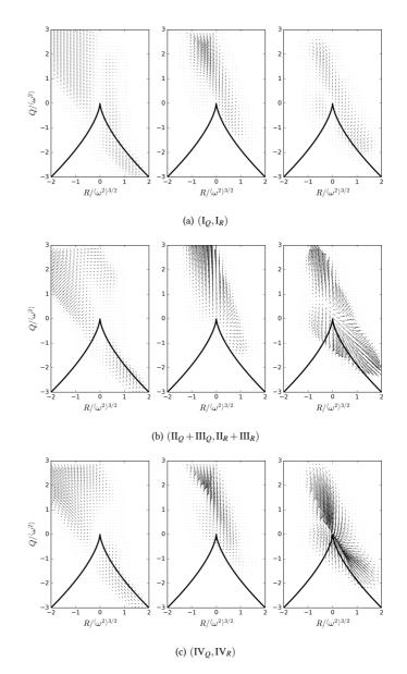
Figure 13. Contributions I (a), II+III (b), and IV (c) to the CMV as given by the LEE for Q and R (case F1). Left column: c < 0.01 (fresh reactants), middle column: 0.01 < c < 0.50, right column: 0.50 < c < 0.95.
