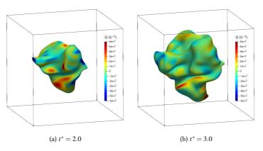
Figure 1. Instantaneous snapshots of the turbulent flame kernels F2 at times  $t^* = 2.0$  (a) and  $t^* = 3.0$  (b): iso-contour c = 0.01 colored by the second invariant Q.
