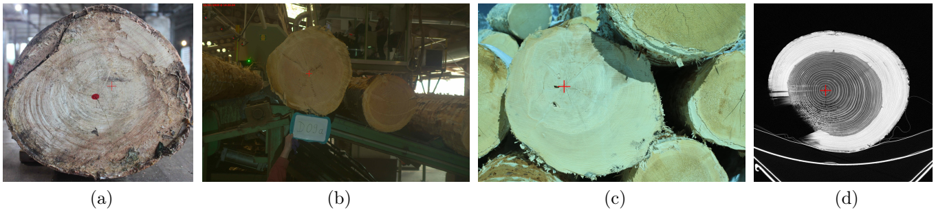
Figure 10: Examples of wood cross-section. Pith estimations by our method are indicated by red crosses.
