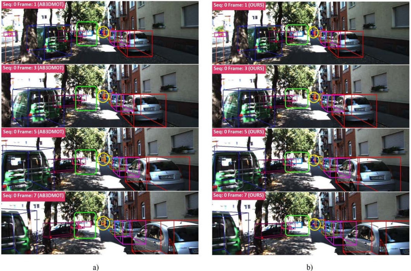
Fig. 5. Qualitative comparison between AB3DMOT [7] (a) and our proposed system (b) on the sequence 0 of the KITTI test set.
