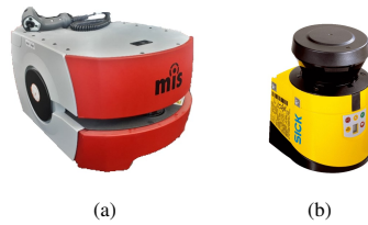
Figure 19: (a) Omron Adept MobileRobots Pioneer LX. (b) SICK LMS 300
