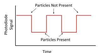
Fig. 2. Representation of the resulting output for the photodiode signal in a low-cost PM sensor using LPO with particles absent (a) and present (b) in the light path.
