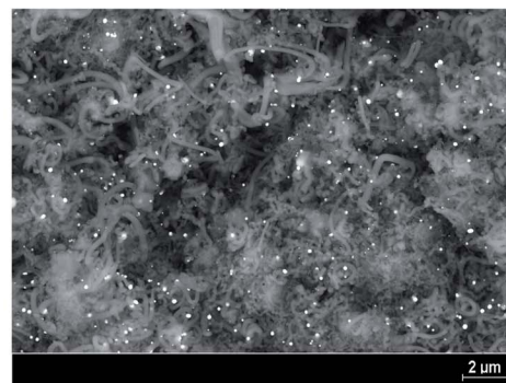
(c) Carbon in the anode outlet pipe.
