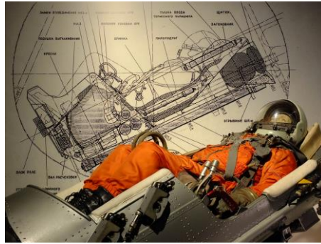
Fig. 1. Vostok ejection seat (licence: Creative Commons).
