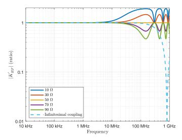
Fig. 6. High-frequency effects  $K^\prime_{HF}$  of inner cable impedance  $Z_{0,inner}$  variation
