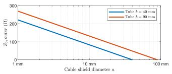
Fig. 3. Characteristic impedance of triaxial tube outer transmission line
