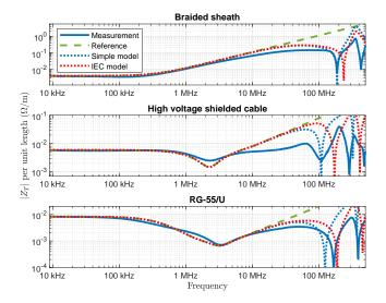
Fig. 12. Comparison of measurement and modeling results with IEC method C in a tube with inner diameter b of 40 mm
