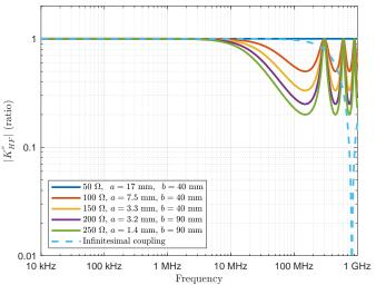
Fig. 5. High-frequency effects  $K_{HF}^{\prime\prime}$  of outer line characteristic impedance  $Z_{0,outer}$  variation with different cable shield and triaxial tube diameters (a and b respectively)
