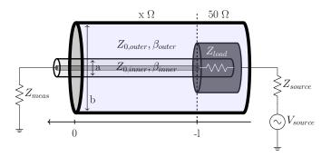
Fig. 1. Drawing of a triaxial tube measurement setup
