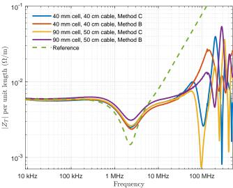
Fig. 10. Transfer impedance measurement results of the high-voltage shielded cable
