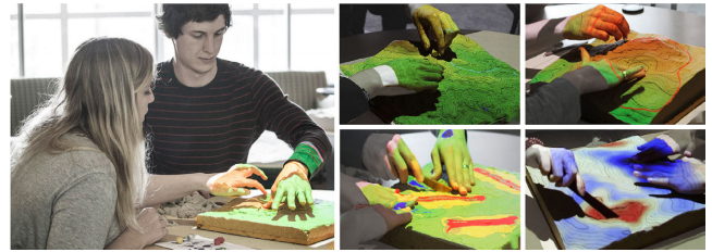
Figure 7: Tangible Landscape is a malleable model, equipped with projectors, that enables users learn about various aspects of topographical properties. Image taken from [MTP*18].
