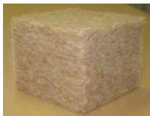
FIG. 1 – Wood/PES fiberboard (100x100x65mm)
