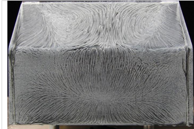
FIG. 5 - Case without control, wall visualization in the base and in the rear window [6].
