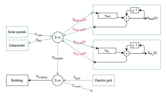
**Figure 1.** View of our system. lines in green shows the solar-only part and purple lines shows the grid-only part. actions are displayed in red.
