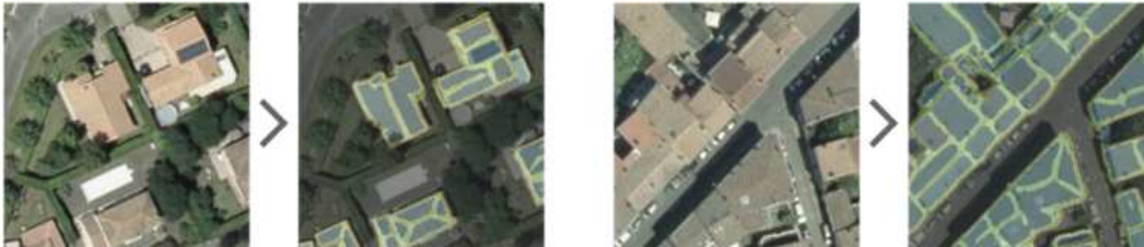
Figure 2: Two examples of aerial image and roof sections semantic segmentation pairs. Sections are depicted in blue, ridges in yellow.
