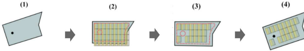
Figure 5: Illustration of the greedy packing algorithm. (1) depicts a roof section containing an object. (2) is the panel packing within the eroded shape after rotating the roof section. (3) shows the best configuration taking into account the margins. (4) depicts the result of the algorithm.
