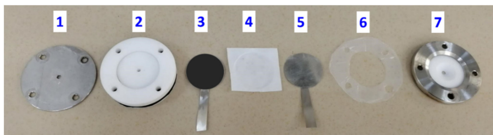
Figure 7. A two-electrode cell: 1—stainless steel plate, 2—polytetrafluoroethylene cell, 3, 5—current collectors (Ni foil), 4—separator (hydrophilic polypropylene membrane), 6—polytetrafluoroethylene isolation gasket, 7—stainless steel cover with polytetrafluoroethylene spacer.
