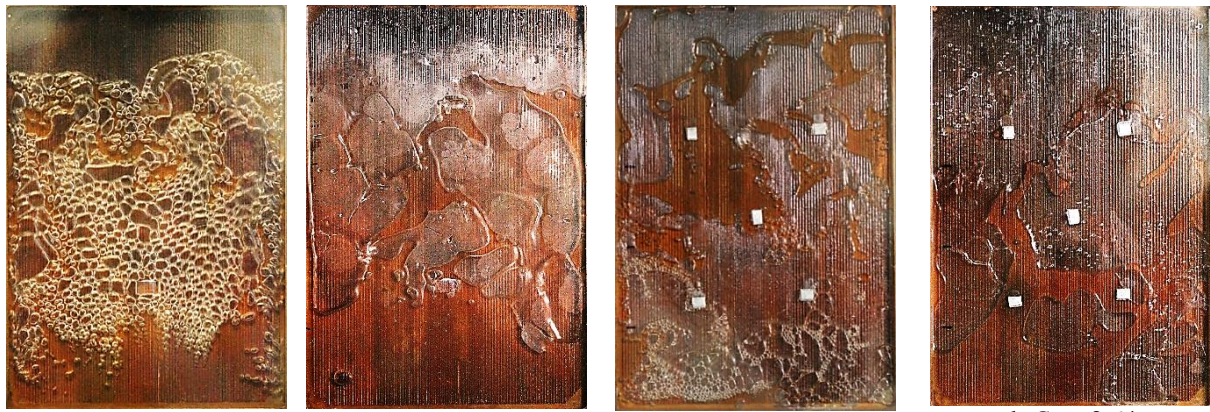
a. Co = 0.54 Pentane, 3 mm, We = 0.14 b. Co = 0.88 Water, 3 mm, We = 0.022 c. Co = 1.62 Pentane, 1 mm, We = 0.25 d. Co = 2.64 Water, 1 mm, We = 0.055 Figure 11: Effect of the confinement for a fixed heat load (100 W, FR = 100\% , \theta = 90^\circ ).
