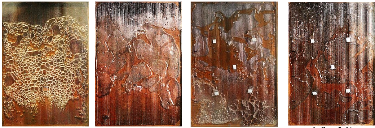
a. Co = 0.54 Pentane, 3 mm, We = 0.14 b. Co = 0.88 Water, 3 mm, We = 0.022 c. Co = 1.62 Pentane, 1 mm, We = 0.25 d. Co = 2.64 Water, 1 mm, We = 0.055 Figure 11: Effect of the confinement for a fixed heat load (100 W, FR = 100\% , \theta = 90^\circ ).
