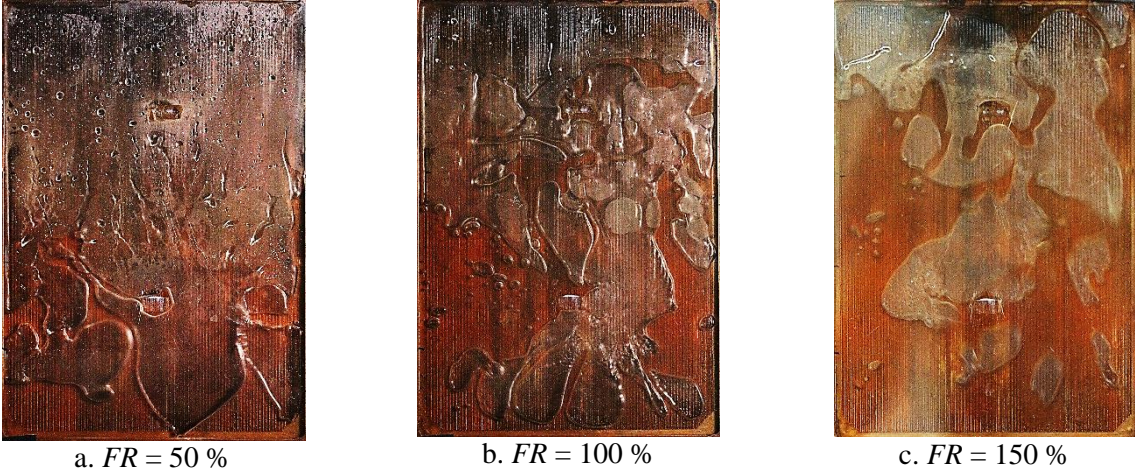
Figure 9: Boiling flow patterns of water at different fill charges. Q = 200W, T_{sink} = 10^{\circ}C, 3\text{ mm. } Co = 0.54, We = 0.12 \pm 15\% .
