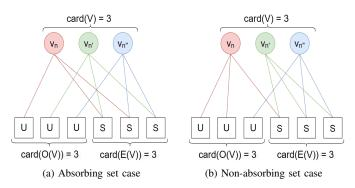
Fig. 1. Example of two sets V, with card(O(V)) = card(E(V)) = 3. If variable-nodes in V are in error, check-nodes marked by an U are unsatisfied, while those marked by an S are satisfied.
