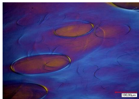
Fig. 2. Image of the surface of BOPP film showing crater-like structure for favoring impregnation
