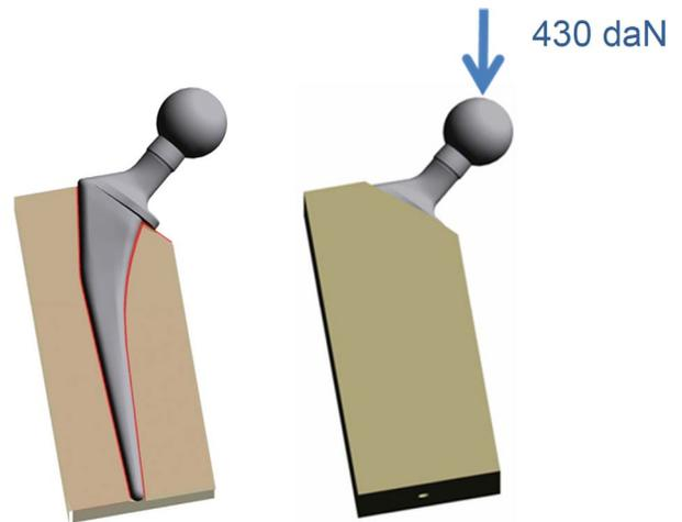
**Figure 2.** Model principle and loading of the stem which is introduced in a bloc with the same mechanical properties as cortical bone.
