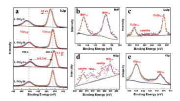
Fig. 5 (a) XPS spectra of Ti2p of different loaded metal oxides. XPS spectra of (b) L-TiO<sub>2</sub>/Bi, (c) L-TiO<sub>2</sub>/Cu, (d) L-TiO<sub>2</sub>/Ni and (e) L-TiO<sub>2</sub>/V.
