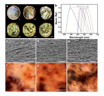
**Fig. 2** (a) Photographs and (b) UV-Vis spectra of CNC/TiO<sub>2</sub> hybrid films. SEM images of CNC/TiO<sub>2</sub> hybrid films: (c) weight ratio=0.5, (d) weight ratio=1.5, (c) weight ratio=2.5 (scale bar = 1  $\mu$ m). POM images of CNC/TiO<sub>2</sub> hybrid films: (f) weight ratio=0.5, (g) weight ratio=1.5, (h) weight ratio=2.5 (scale bar = 50  $\mu$ m).
