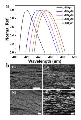
**Fig. 4** (a) UV-Vis spectra and (b) SEM images of CNC/loaded metal oxide hybrid films (scale bar = 1 µm).
