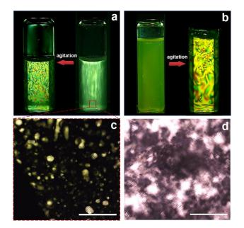
**Fig. 1** Photographs of (a) pure CNC and (b) TAA/CNC (weight ratio=0.5) suspensions observed between crossed poalrizers before and during agitation (shear-induced polychromatic birefringence). Typical POM images of (c) CNC and (d) TAA/CNC suspensions during slow evaporation at room temperature (scale bar = 50 μm).
