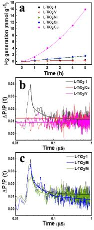
Fig. 6 (a) Hydrogen generation of metals loaded lamellar  $TiO_2$  films. TRMC signals of (b) L-TiO<sub>2</sub>/Cu and L-TiO<sub>2</sub>/V, (c) L-TiO<sub>2</sub>/Bi and L-TiO<sub>2</sub>/Ni.
