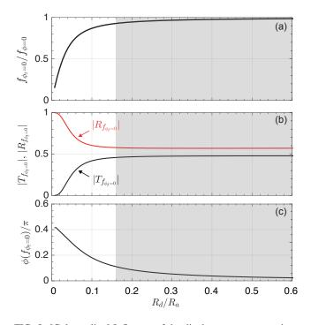
FIG. 5. [Color online] Influence of the diaphragm aperture ratio on its scattering parameters (analytically calculated).
