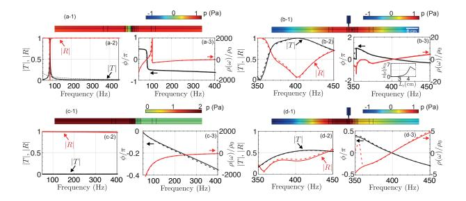
FIG. 3. [Color online] (a,c) Cloaking of a  $R_d = 0.15$  mm diaphragm in a conventional 6 PAM: lossless (a) and lossy (c) configurations. (b,d) Cloaking of a  $R_d = 4$  mm diaphragm in a 6 PAM doped with a Helmholtz resonator ( $R_n = 2$  mm,  $L_n = 2$  cm,  $R_c = 1$  cm, and  $L_c = 40.95$  cm): lossless (b) and lossy (d) configurations.
