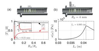
FIG. 2. [Color online] Geometry optimization from analytical formulas for cloaking a diaphragm using a 6-unit long lossless PAM: (a) sketch of the configuration and influence of the diaphragm radius on the system's scattering parameters, (b) sketch of the configuration with an external dopant and optimal geometry for cloaking by doping a 6-unit long lossless PAM with a Helmholtz resonator. Evolution of the effective bulk modulus with the cavity length of the Helmholtz resonator.
