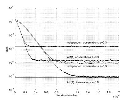
Figure 6: Learning curves of  $E \| \mathbf{P}_k - \mathbf{P}_* \|_{Fro}^2$  compared to  $\gamma \text{Tr}(\mathbf{C}_P)$  averaging 100 independent runs for real independent or AR(1) learning patterns and for the parameter a = 0.3 and a = 0.9 for the SNL algorithm with  $\gamma = 0.005$ .
