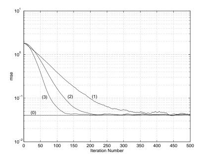
Figure 1: Learning curves of the mean square error  $E \| \mathbf{P}_k - \mathbf{P}_* \|_{Fro}^2$ , averaged over 100 independent runs, for the SNL algorithm (1), and the smoothed SNL algorithm for the following different values of the parameter  $\alpha$ :  $\alpha = 1$  (2),  $\alpha = 0.3$  (3), compared to the theoretical value  $\gamma \text{Tr}(\mathbf{C}_P)$  (0).
