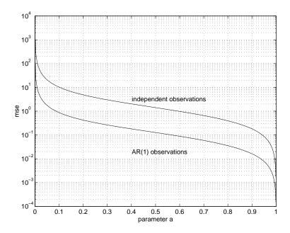
Figure 7: Mean square error of the projection matrix (normalized by the gain factor  $\gamma$ ) on the eigenspace generated by the first two eigenvectors for independent or AR(1) consecutive learning patterns  $\mathbf{x}_k$  for the same covariance matrix  $\mathbf{R}_x$  as a function of the parameter a.
