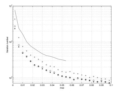
Figure 5: Iteration number until "convergence" is achieved, versus theoretical asymptotic mean square error  $\gamma \text{Tr}(\mathbf{C}_P)$ , of the SNL algorithm (-), and of the smoothed SNL algorithm with  $\alpha = 1$  (+),  $\alpha = 0.2$  (\*) and  $\alpha = 0.3$  (o).
