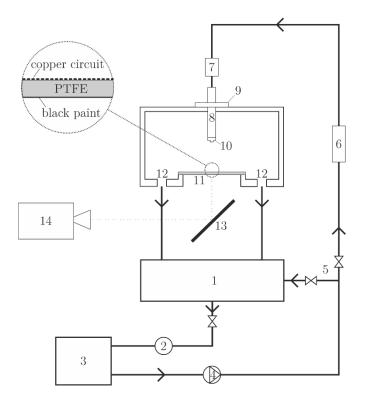
*Fig. 1.* Schematic view of the experimental apparatus for thermal measurements: (1) tank; (2) filter; (3) thermostat; (4) gear pump; (5) bypass; (6) ultrasound flow-meter; (7) platinum resistance thermometer; (8) nozzle holder; (9) nozzle adjustment collar; (10) nozzle; (11) target plate; (12) evacuation channel; (13) golden mirror; (14) infrared thermal camera
