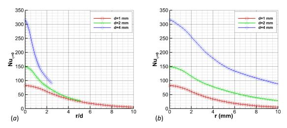
Fig. 10. Illustration of local Nusselt number dependence on injection diameter (normalized distance (a) and non-normalized distance (b) from stagnation point). Pr = 328, Re = 660, z/d = 10
