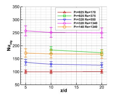
Fig. 11. Stagnation Nusselt number for three different nozzle-to-target distance and various Reynolds and Prandtl number couples. d = 2 mm
