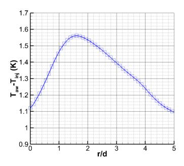
*Fig. 3.* Radial variation of the temperature difference of adiabatic wall temperature to injection temperature. Pr = 737, Re = 660, d=2 mm, z/d = 10
