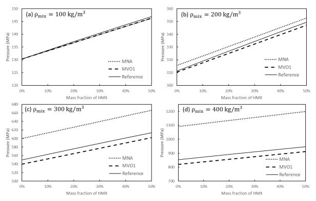
**Figure 8.** Closed bomb vessel pressure for various mixtures of NC-13 and HMX. The black solid line represents reference results obtained with the thermochemical code CHEETAH. The black dotted line represents the MNA EOS results. The black dashed line represents the MVO1 EOS results. Pressures are computed for different loading densities {100 ; 200 ; 300 ; 400} kg/m<sup>3</sup>. As before, better agreement is obtained with MVO1 than MNA, especially when extrapolating at higher densities.
