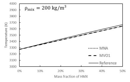
**Figure 7.** Flame temperature for various mixtures made of NC-13 and HMX at loading density 200 kg/m<sup>3</sup>. The black solid line represents reference results obtained with the thermochemical code CHEETAH. The black dotted line represents the MNA EOS results. The black dashed line represents the MVO1 EOS results. Predictions for both reduced mixture EOS are identical and very close to the reference.
