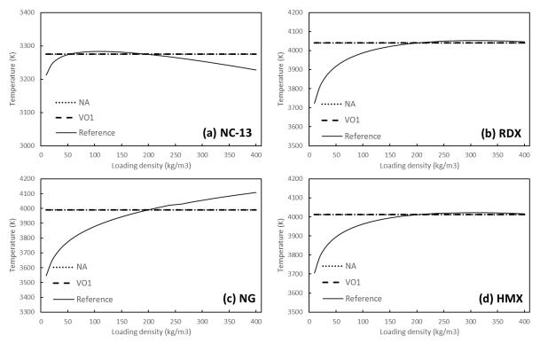
**Figure 1.** Flame's temperature of various reactive materials computed for different loading densities. Reduced NA and VO1 EOS are compared to CHEETAH computations, considered as reference. The black solid line represents the reference results. The black dotted line represents the NA EOS results. The black dashed line represents the VO1 EOS results. Both reduced EOS predictions are identical and equal to the flame temperature used in parameters determination (Table I).
