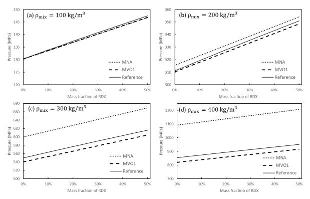
**Figure 6.** Closed bomb vessel pressure for various mixtures of NC-13 and RDX. The black solid line represents reference results obtained with the thermochemical code CHEETAH. The black dotted line represents the MNA EOS results. The black dashed line represents the MVO1 EOS results. Pressures are computed for different loading densities {100 ; 200 ; 300 ; 400} kg/m<sup>3</sup>. As before, better agreement is obtained with MVO1 than MNA, especially when extrapolating at higher densities.
