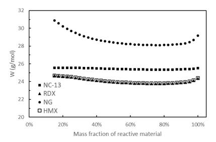
**Figure 9.** Molar mass of gas products resulting of reactive material combustion in inert Argon, computed with the thermochemical code CHEETAH for various mass fraction of reactive material. Considered materials are NC-13 in black filled squares, RDX in black filled triangles, NG in black filled circles and HMX in black empty squares. RDX and HMX results are merged.
