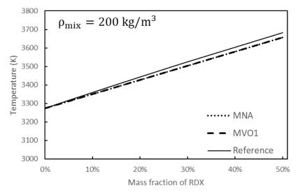
**Figure 5.** Flame temperature for various mixtures made of NC-13 and RDX at loading density 200 kg/m<sup>3</sup>. The black solid line represents reference results obtained with the thermochemical code CHEETAH. The black dotted line represents the MNA EOS results. The black dashed line represents the MVO1 EOS results. Predictions for both reduced mixture EOS are identical and very close to the reference.
