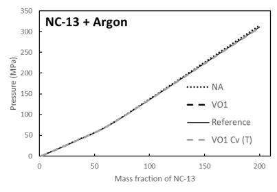
**Figure 4.** Computed pressure comparison in closed bomb vessels for different mixtures of NC-13 and Argon. The black solid line represents reference results obtained with the thermochemical code Cheetah. The black dotted line represents the NA EOS results. The black dashed line represents the VO1 EOS results with constant specific heat. The grey dashed line represents VO1 EOS results with variable specific heat. All curves are in very close agreement.
