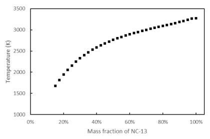
**Figure 10.** Flame temperature of various mixtures made of NC-13 and Argon. These mixtures are used in system (C.5) to determine parameters of the combustion products temperature dependent specific heat.
