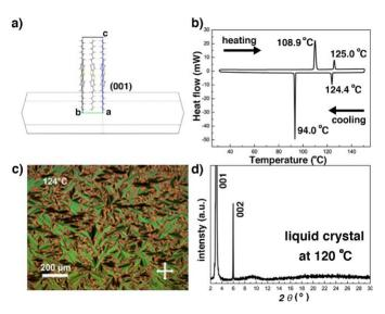
**Fig.2** (a) Predicted crystal morphology of C8-BTBT-C8 based on the BFDH method. (b) DSC trace of C8-BTBT-C8. (c) POM picture of the fan shaped texture of the SmA liquid crystal phase of C8-BTBT-C8 recorded at 124 °C. (d) sXRD pattern of the SmA phase recorded at 120 °C.
