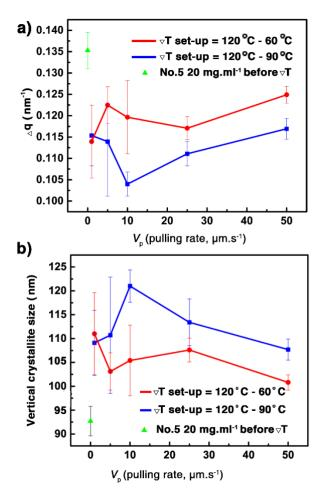
**Fig. 6** Evolution of the FWHM of the (002) Bragg peaks of the samples(a) and the vertical crystallite size of films  ${\bf 10}-{\bf 19}$  as a function of the pulling rate ( $V_p$ ) for two  $T_h-T_c$  couples (b). The data of just coated film  ${\bf 5}$  are shown for comparison. See also in Table  ${\bf 53}$ .
