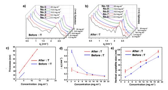
Fig. 4 XRR curves of the C8-BTBT-C8 thin films (1-10) before (a) and after (b) the  $\nabla T$  treatment, recorded at room temperature. Evolution of the film thicknesses (c), the FWHM of the (002) Bragg peaks (d), and the vertical crystallite size (e) as a function of the solution concentrations before and after the  $\nabla T$  treatments. See also Table **S2**.
