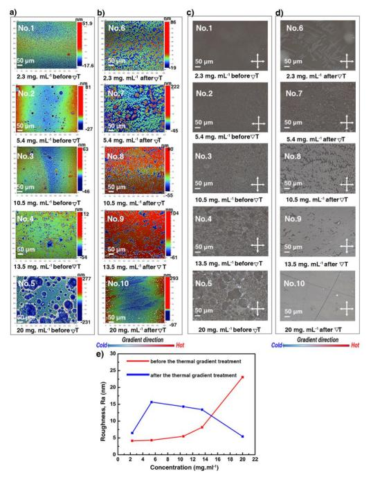
Fig. 3 Surface morphology of the C8-BTBT-C8 spin-coated thin films produced using different solution concentrations before: a) optical profilometry images and c) POM images; and after the ∇T treatment; b) optical profilometry images and d) POM images, recorded at room temperature. The gradient direction is highlighted (bottom). e) Evolution of the film surface roughness (Ra) as a function of the solution concentration. See also Table **S2**.
