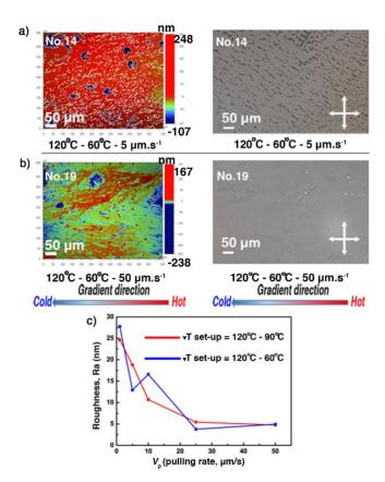
**Fig. 5** The surface morphology (optical profilometry and POM images) of the C8-BTBT-C8 thin films **14** (a) and **19** (b) presents the features of partial or complete covering of the glass substrate. Pictures were recorded at room temperature. The gradient direction is highlighted (bottom). (c) Evolution of the film surface roughness (Ra) as a function of the pulling rate ( $V_p$ ) for different  $T_h$  -  $T_c$  couples. See also Table **S3**.
