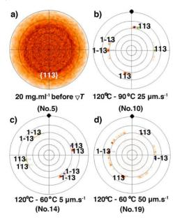
**Fig.7** (a) Pole figure of {113} reflections for the spin-coated film **5** before the  $\nabla T$  treatment. Pole-figure measurements of {113} reflection for films **10** (b), **14** (c) and **19** (d), after the  $\nabla T$  treatments. The black solid dot highlights the temperature gradient direction.
