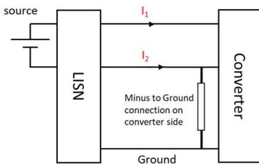
Fig. 6. Validation case "Minus to ground". The minus of the converter is connected to the ground through an almost zero impedance (actually 5 nH – 265 m $\Omega$ ). The LISN minus is not connected to the ground.
