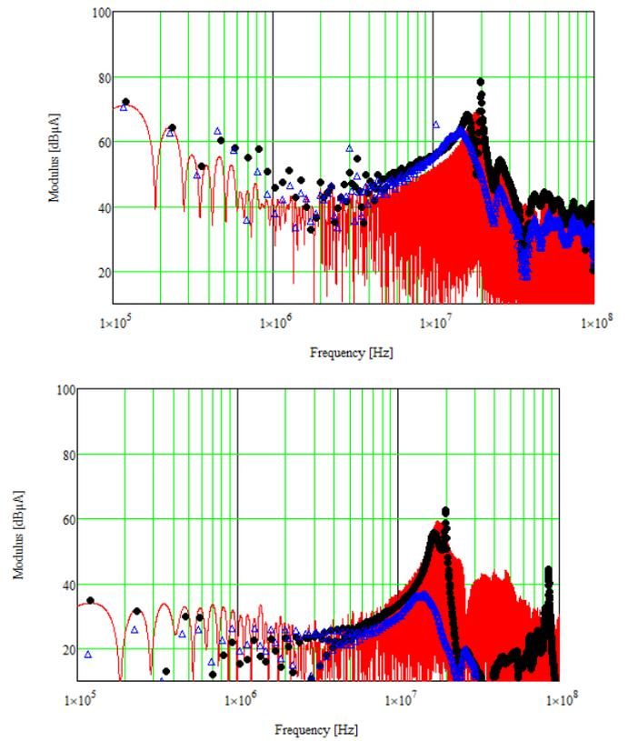
Fig. 14. Comparison between asymmetric frequency model (black points), symmetric frequency model (blue points) and measurement (red) for minus to ground test case (Top I<sub>1</sub>, Bottom I<sub>2</sub>)
