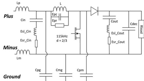
Fig. 7. Equivalent circuit of the Boost converter used for simulation.
