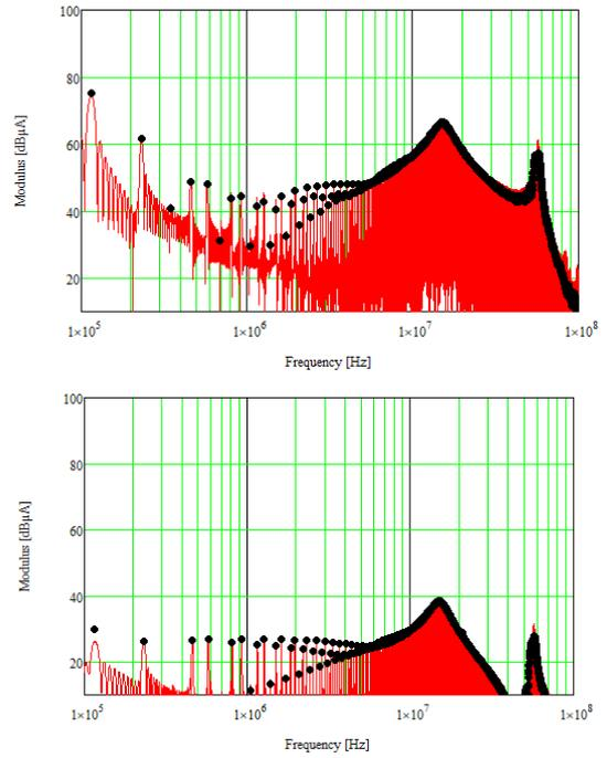
Fig. 9. Comparison between frequency model (black points) and time domain simulation + FFT (red) for minus to ground (Top  $I_1$ , Bottom  $I_2$ )
