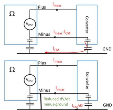
Fig. 4. Reducing potential CM circulation when connecting the impedance bridge to the ground.
