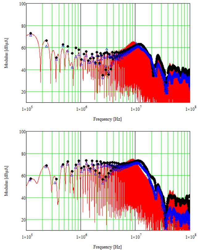
Fig. 15. Comparison between asymmetric frequency model (black points), symmetric frequency model (blue points) and measurement (red) for asymmetric LISN test case (Top I<sub>1</sub>, Bottom I<sub>2</sub>)
