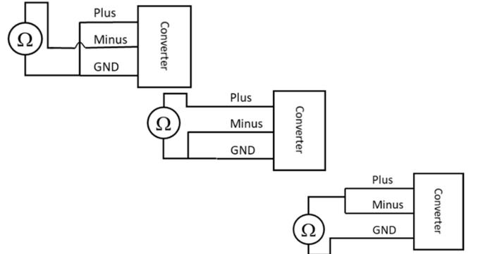
Fig. 3. The 3 impedance measurement configurations to identify the three impedances of the model. Top:  $Z_{PG}$  with Plus and Ground connected, Middle:  $Z_{MG}$  with Minus and Ground connected, Bottom:  $Z_{PM}$ , with Plus and Minus connected.
