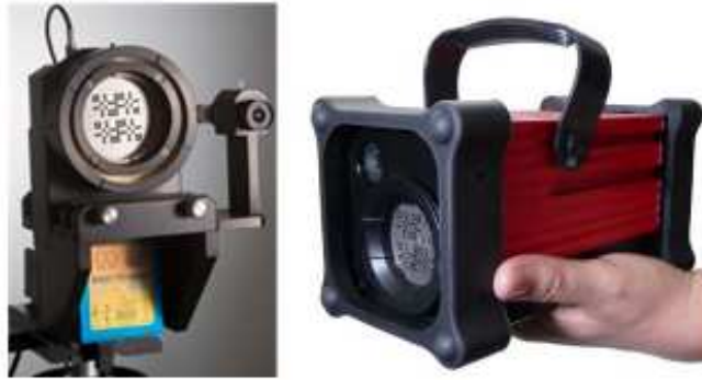
Fig 1. On the left: GAMPIX gamma camera prototype developed by CEA LIST. On the right: the industrial iPIX version commercialized by Mirion Technologies (CANBERRA).
