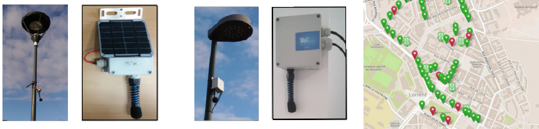
Figure 2 - The leaf (left) and gateway (middle) sensors. Right: Deployment in the City of Lorient
