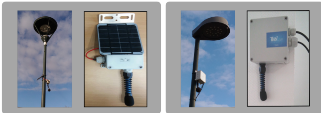
Fig. 2: The leaf (left) and gateway (right) sensors.
