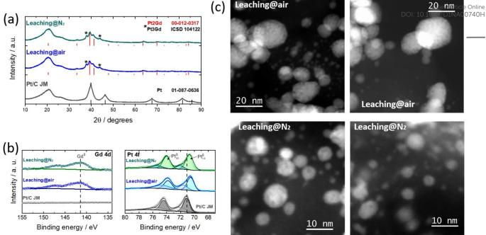
Fig. 1 (a) Powder XRD patterns; (b) Gd 4d and Pt 4f photoemission lines; and (c) high-angle annular dark field STEM micrographs of the Pt<sub>v</sub>Gd/C catalysts washed under air- or N<sub>2</sub>-atmosphere. 40% Pt/C from Johnson-Matthey is used as reference in (a) and (b).
