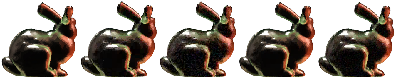
Fig. 8: Comparing reconstructions of Bunny from Fig. 7 at viewpoint arrangement 16x8, at similar bitrates for 6-D RAHT and RAHT-KLT, using an angular rescaling of 0-511 for 6-D RAHT. Left to right: Input, 6-D RAHT reconstruction at 0.7 bpp and PSNR 30.8 dB, RAHT-KLT reconstruction at 0.8 bpp and PSNR 25.4 dB, 6-D RAHT reconstruction at 1.4 bpp and PSNR 41.6 dB, RAHT-KLT reconstruction at 1.4 bpp and PSNR 30.7 dB.
