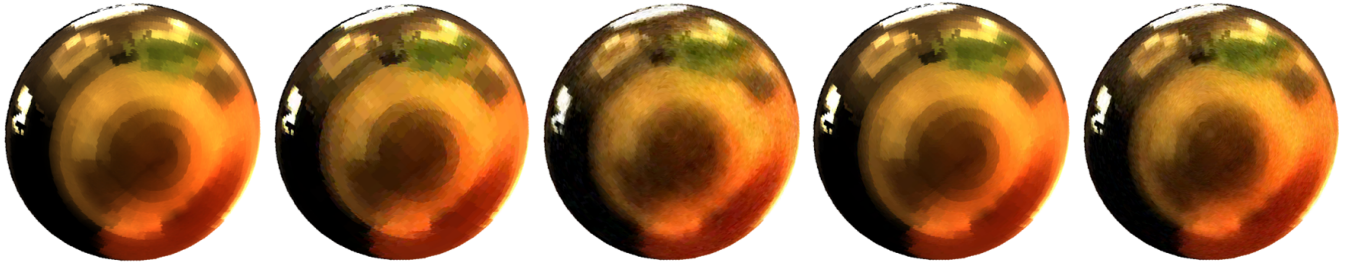
Fig. 11: Comparing reconstructions of Gold Sphere from Fig. 10 at viewpoint arrangement 32x16, at similar bitrates for 6-D RAHT and RAHT-KLT, using an angular rescaling of 0-1023 for 6-D RAHT. Left to right: Input, 6-D RAHT reconstruction at 0.4 bpp and PSNR 33.2 dB, RAHT-KLT reconstruction at 0.5 bpp and PSNR 26.1 dB, 6-D RAHT reconstruction at 1.0 bpp and PSNR 41.7 dB, RAHT-KLT reconstruction at 1.1 bpp and PSNR 30.4 dB.
