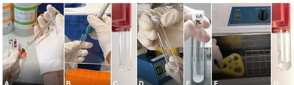
Figure 2. Workflow for the production of phospholipid vesicles. A. Put phospholipids in a glass tube using a Hamilton syringe. B. Evaporate chloroform using argon or nitrogen gas. C. Evaporated
