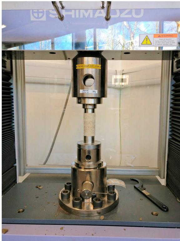
Figure 1. Unconfined compression test setup.
