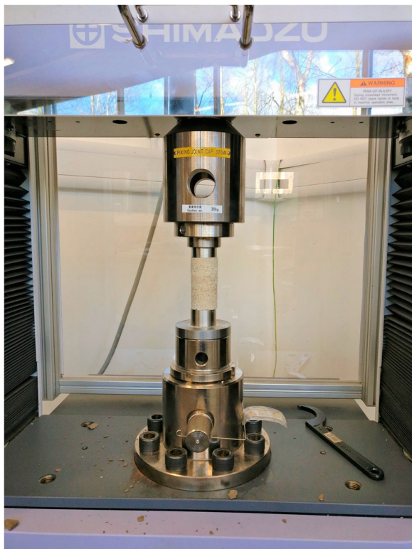
Figure 1. Unconfined compression test setup.
