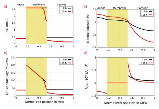
**Fig. 6.** Calculated profiles of IEC (a), hydroxide conductivity (b), electric potential in the ionomeric phase (c) and reaction rate distribution (d) across the cell at different times (0 and 105 h) after starting AEMFC operation at 0.6 A/cm<sup>2</sup>. The origin of the x-axis corresponds to the anode CL –GDL interface.
