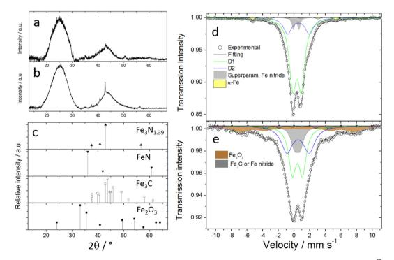
**Fig. 1.** Structural characterization of  $Fe_{0.5}$ -dry and  $Fe_{0.5}$ -hydrate. XRD patterns for a)  $Fe_{0.5}$ -dry and b)  $Fe_{0.5}$ -hydrate. c) XRD patterns for reference compounds. <sup>57</sup>Fe Mössbauer spectra for d)  $Fe_{0.5}$ -dry and e)  $Fe_{0.5}$ -hydrate. For c), the most intense diffraction peaks are represented for  $Fe_3N_{1.39}$  (JCPDS file 04-023-4686, FeN (00-050-1087),  $Fe_3C$  (00-034-0001) and  $Fe_2O_3$  (00-033-0664). Mössbauer spectra were acquired at 5 K.
