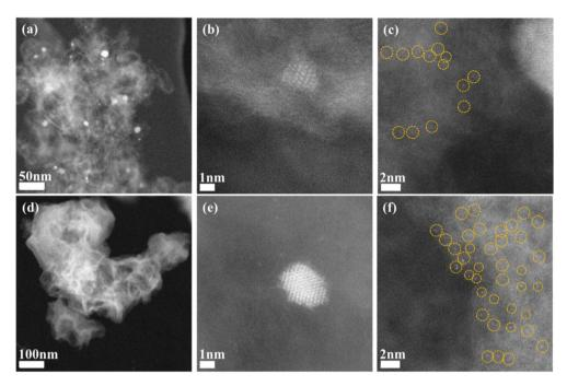
**Fig. 2.** ADF-STEM images of  $Fe_{0.5}$ -hydrate and  $Fe_{0.5}$ -dry. Images of  $Fe_{0.5}$ -hydrate showing (a) large Fe particles with different sizes, (b) small Fe particle with no single Fe atom around the particle, (c) some single Fe atoms away from sintered particles, and images of  $Fe_{0.5}$ -dry (d) showing no large Fe particles, (e) nanoparticle with several single Fe atoms nearby, (f) single Fe atoms dispersed on the carbon support.
