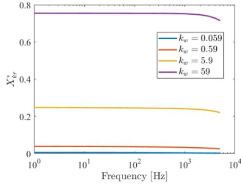
**Fig. 8.** Effect of the thermal conductivity  $k_w$  of the surrounding material on the sensitivity coefficient of the fiber temperature with respect to its radial thermal conductivity  $k_r$
