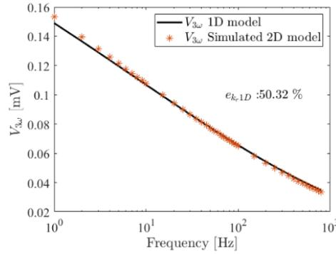
**Fig. 6.** Computation of the bias  $e_{kr1D}$  on the estimated radial conductivity by using the 1D analytical model (simulated data using the 2D analytical model with  $k_z = 10 \text{ Wm}^{-1}\text{K}^{-1}$  and  $k_r = 1 \text{ Wm}^{-1}\text{K}^{-1}$ )
