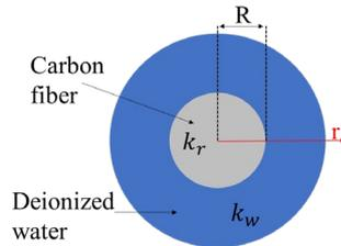
**Fig. 2.** Geometry for the 1D thermal model with a carbon fiber surrounded by de-ionized water
