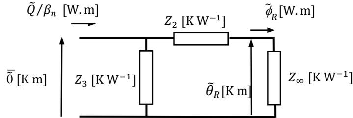
**Fig. 4.** Representation of the 2D thermal model using impedances
