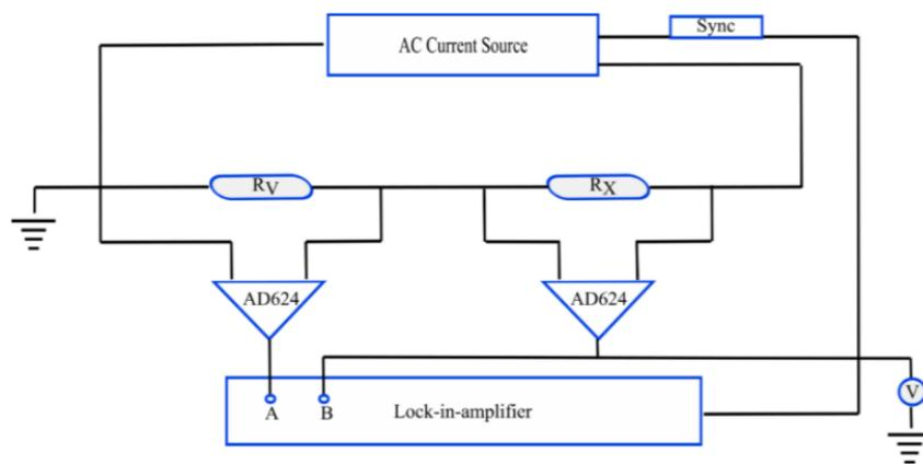
**Fig. 9.** Schematic electrical setup for  $3\omega$  voltage measurement.
