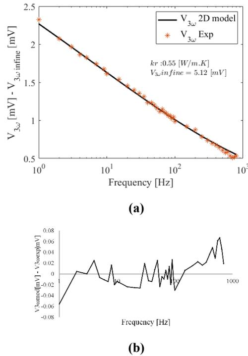
**Fig 11. (a)** Measured and computed  $V_{3\omega}$  voltages after the estimation of the radial thermal conductivity (sample#1, FT300B carbon fiber) **(b)**  $V_{3\omega}$  residuals
