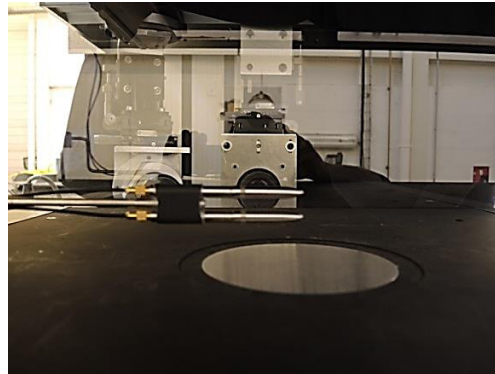
Figure 6. Picture of a plain panel flush-mounted on the base wall of the wind-tunnel test section
