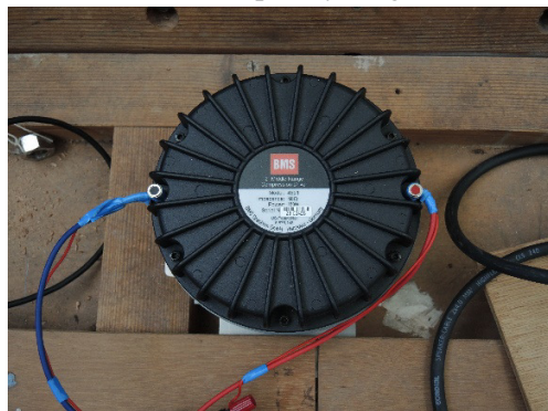
Figure 4. Photography of the acoustic compression driver mounted on the wind tunnel wall
