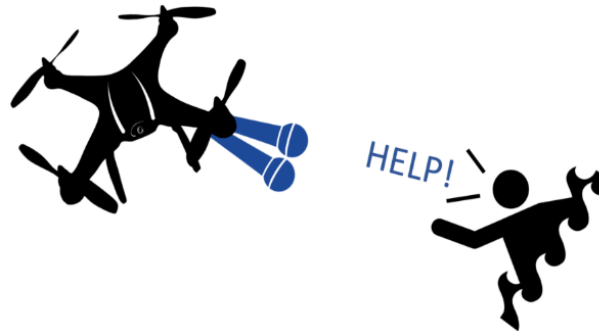
Figure 1: Microphones embedded in a drone may help localizing people for search and rescue in disaster area.
