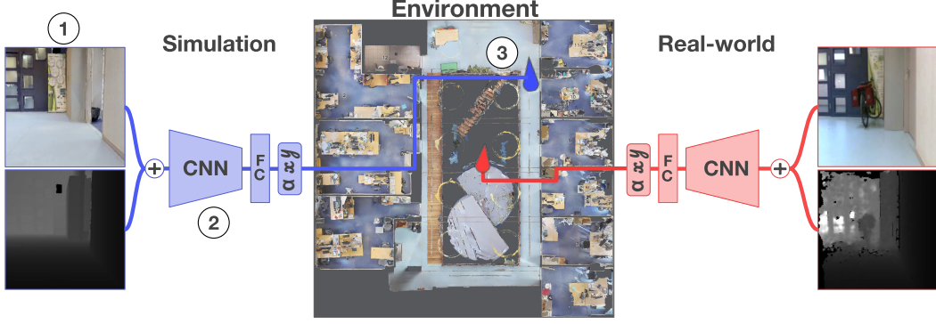
Figure 2: In the studied robot ego-localization task, an RGB-D image ①, is given to a trained model ②, which uses it to regress the location (x, y) , and orientation angle (\alpha) in the environment from which this image was taken from ③. As illustrated above, images taken from the same coordinates in simulation and real-world ① may lead to different predictions due to differences, such as here, among others, the additional presence of a bike in the scene. We are interested in reducing the gap between the SIM and REAL predictions.
