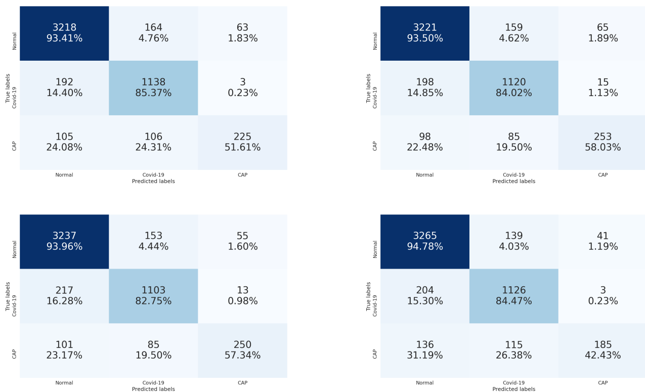
Figure 7. Confusion matrices of the stacked grayscale image and the segmented lung lobes on validation data using ResneXt-50, Densenet-161, Inception-v3, and Wide-Resnet-50, respectively. The vertical axis is for the true classes, and the horizontal axis is for the predicted classes.
