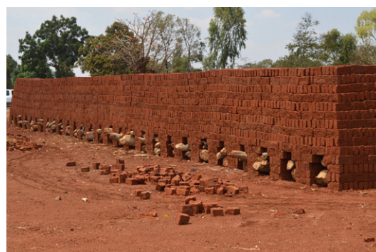
High capacity clamp in Benga, Mchinji. © Jon Twingi.
