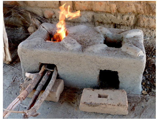
Changu Changu Moto stove is one of the several models of improved stoves existing in Malawi. The stove reduces wood usage, there is less risk of burns and smoke inhalation and two things can be cooked at the same time on the two burners. © Ripple Africa
