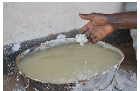
Lime is used for the whitewashing of earth constructions and also mixed with earth for plastering. Iuluma, Chitipa. © Jon Twingi.
