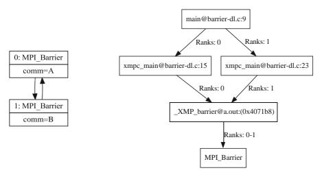
Fig. 2 Deadlock detected by MUST for Listing 3 when only looking at MPI
