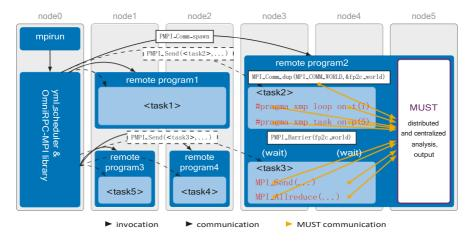
**Fig. 6** Integration of MUST into FP2C: the YML scheduler launches selected YML tasks under the control of MUST runtime correctness checking. MUST analyses are applied only to parallel programming constructs used in the task code, but not to MPI communication utilized by the FP2C command and control workflow
