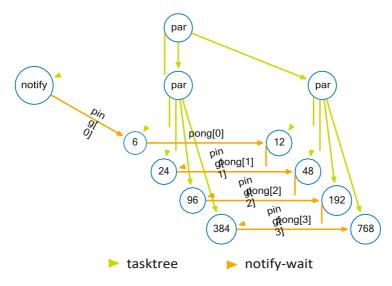
Fig. 3 Graph of tasks as defined by the YvetteML code in Listing 6. The task nodes representing the inner task executing the compute add are represented by the result of their computation
