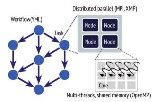
Fig. 1 An overview of multi-SPMD programming model
