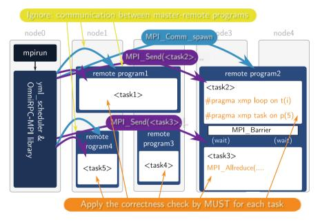
Fig. 17 Applying MUST to the mSPMD programming model. Only communication functions written in red letters are checked, MPI functions written in black letters are not checked
