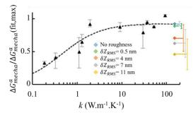
Fig. 4. Normalized thermal conductance across contact as a function of apparent sample thermal conductivity *k* for both reference and rough samples (Pd probe operated in vacuum). The dashed black line is a calibration curve obtained from average thermal conductances of bulk reference materials with roughness as low as possible (black dots) with a different probe (see Suppl. Mat. for explanations).
