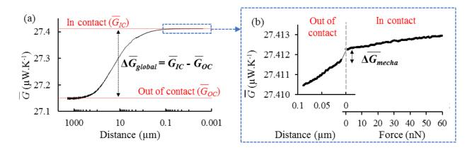
FIG. B. Thermal conductance of the probe-sample system  $\overline{G}$  as a function of distance to contact with a flat Si reference sample (DS probe in air). (a) Thermal conductances  $\Delta \overline{G}_{global}$  including all heat transfer channels and (b)  $\Delta \overline{G}_{mecha}$  at the contact jump and as a function of the probe-sample force.
