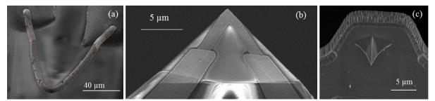
FIG. A. SEM images of (a) the Wollaston probe, (b) the Pd probe and (c) the DS probe.
