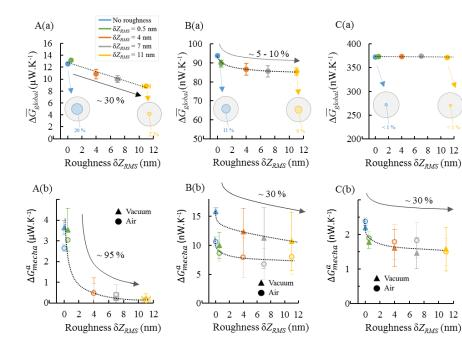
contact-related (b) thermal conductances according to the Si roughness, for the Wollaston (A), Pd (B) and doped Si (C) probes. Figs. (a) refer only to air measurements. Inset represent schematics the percentage of the mechanical contact heat transfer in the global heat transfer between probe and sample. For vacuum measurements  $\Delta \bar{G}_{global} = \Delta G^a_{mecha}$
