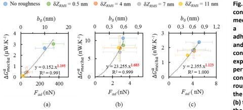
3. Thermal conductance due to mechanical contact as function of the adhesion force (Fad) and corresponding contact radii for experiments performed in air conditions on the rough samples with (a) the Wollaston probe, (b) the Pd probe and (c) the DS probe.
