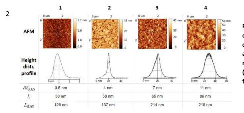
Fig. 1. Topographic images obtained from AFM, distributions of the associated heights and roughness parameters (δZ<sub>RMS</sub>, l<sub>c</sub> and L<sub>RMS</sub>) for the four rough samples
