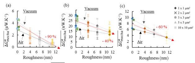
Fig. D. Thermal conductance  $\overline{\Delta G^a_{mecha}}$  estimated from images of rough Si samples with different areas (ambient and vacuum conditions) with the (a) Wollaston, (b) Pd and (c) DS probes.
