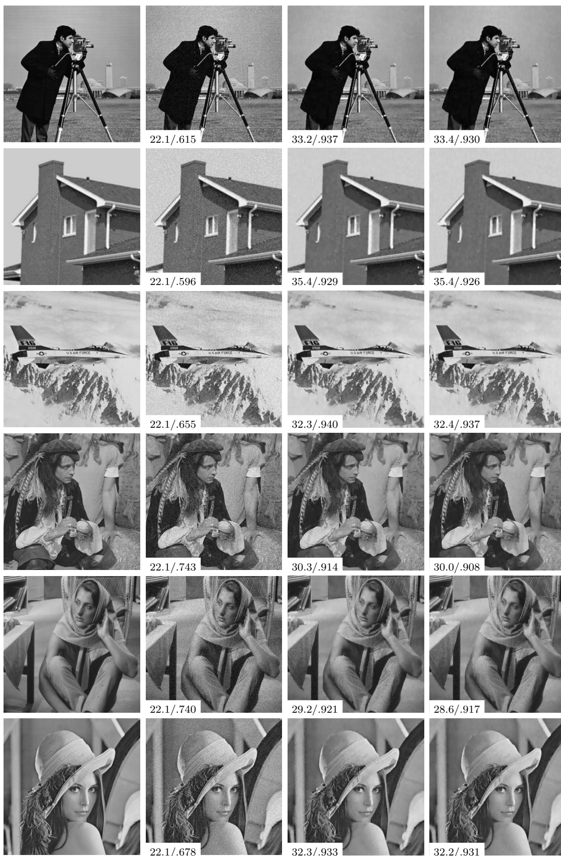
Figure 4. From left to right: Original images, noisy images with noise \sigma = 20 , results with EM model, results with LR-COMP model. The denoising results are evaluated with PSNR/SSIM. Similar denoising performances are obtained with LR-COMP with a 1000 times smaller compressed database. To estimate the prior model, our method is 2 times faster than the EM algorithm.
